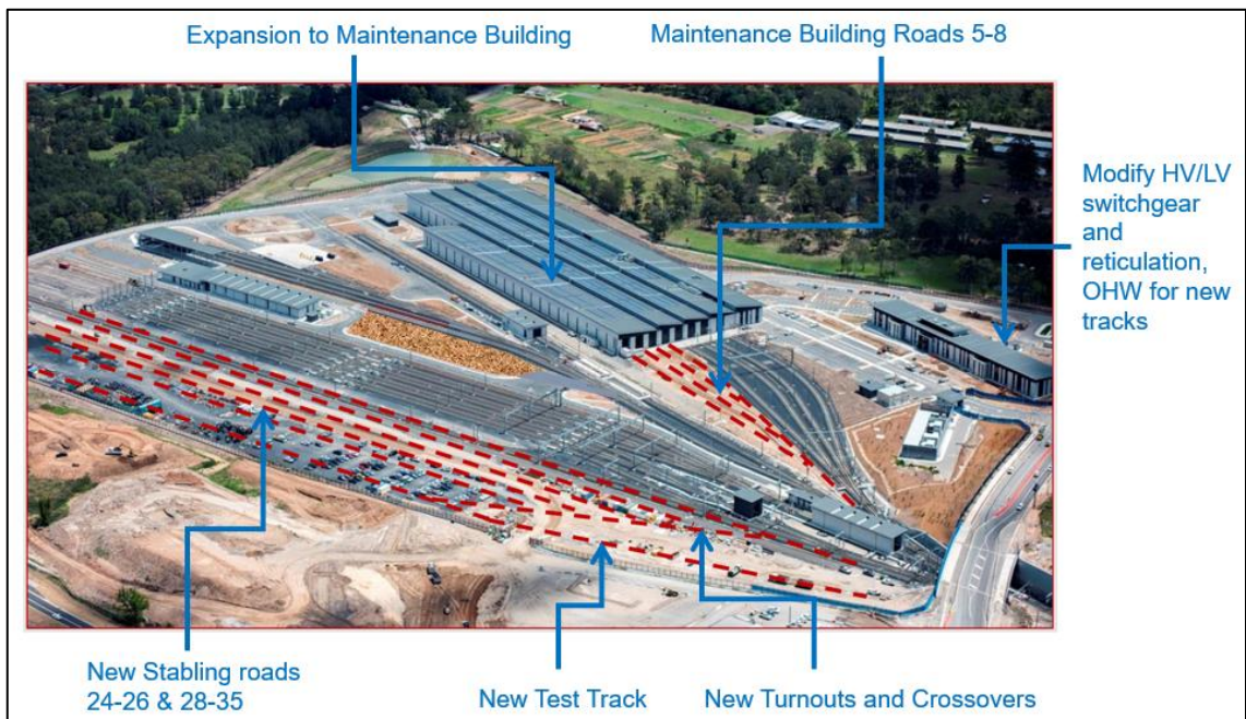
Figure 3: SMTF Expansion Scope of Work
